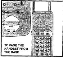
This feature is also useful if you have misplaced the handset. To locate the handset press **PAGE** at the base. This starts a paging tone at the handset. When it is located, cancel the paging tone by pressing **OFF** on the handset.
